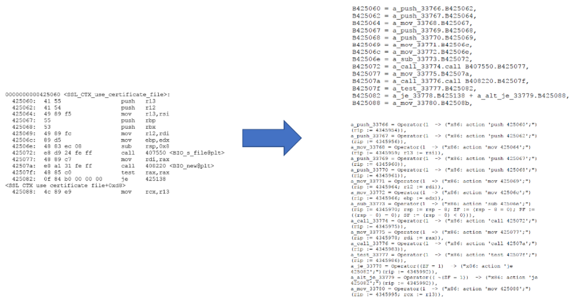
Figure 2: Translation of assembler x86 code to algebraic specifications
