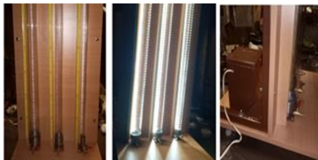
Figure 5: Laboratory installation for determining the coefficient of dynamic viscosity of the liquid by the Stokes method
