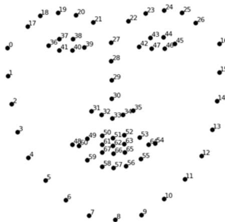
Figure 1: Landmark points of the human face recognized by the OpenCV library
